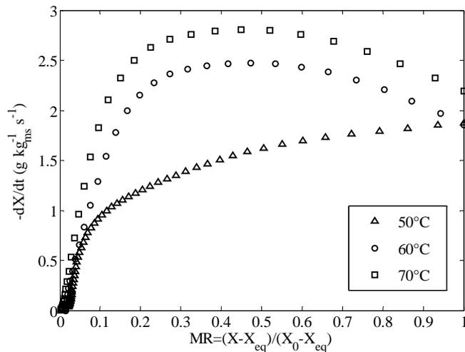
**Figure 3:** Influence of temperature on the drying rate of Amelie mango slice
