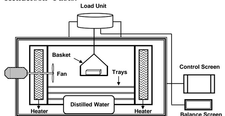
**Figure 1:** Schematic illustration of the experimental dryer set-up.
