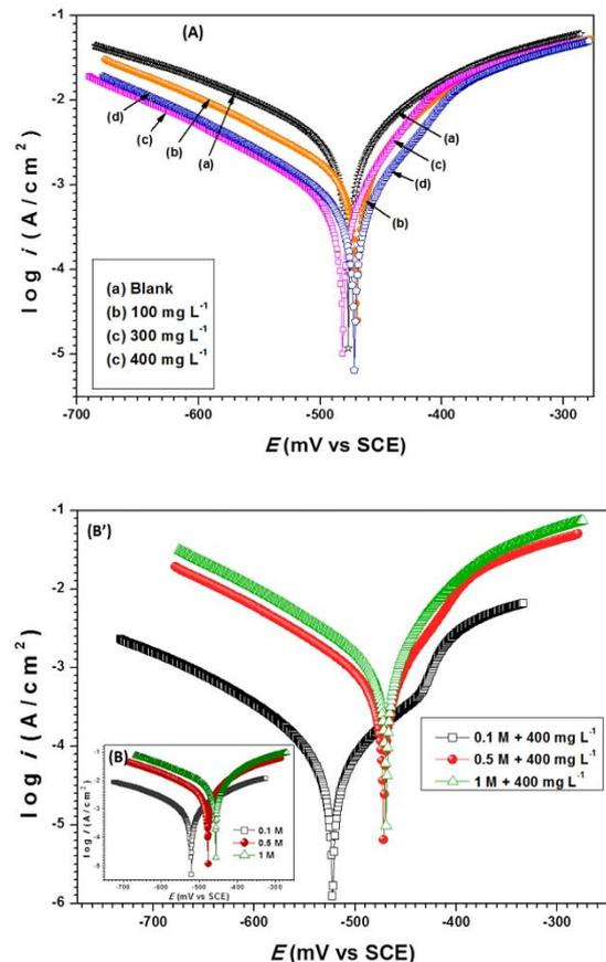
**Figure 4:** Tafel curves of carbon steel immersed in (A) 0.5 M H<sub>2</sub>SO<sub>4</sub> without and with different concentration of MELE at 30°C and (B, B') influence of acid concentration
