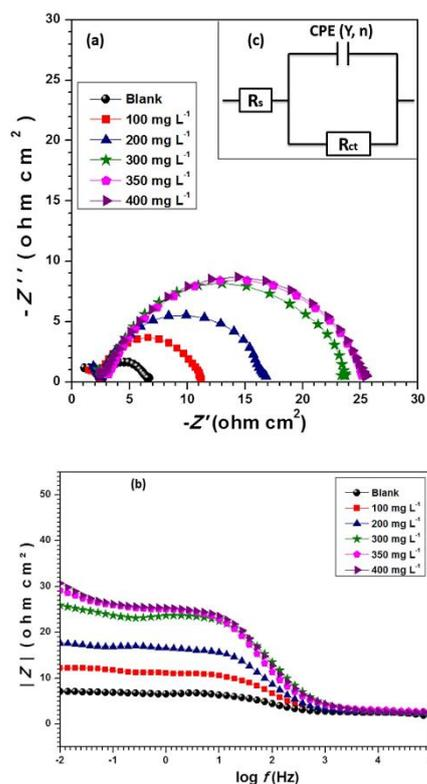
**Figure 5:** Electrochemical impedance spectra: (a) Nyquist and (b) Bode plots, and (c) equivalent circuit proposed for the metal / electrolyte interface
