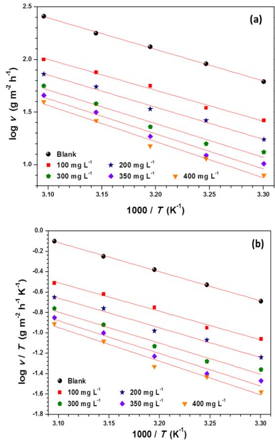
**Figure 9:** Plots of Arrhenius for carbon steel immersed in 0.5 M H<sub>2</sub>SO<sub>4</sub> without and with MELE: (a)  $\log v$  as a function of  $1000/T$  and (b)  $\log v/T$  as a function of  $1000/T$
