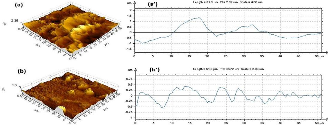
**Figure 7:** AFM image of the carbon steel after 1 hour of immersion in 0.5 M H<sub>2</sub>SO<sub>4</sub> (a) without and (b) with 400 mg L<sup>-1</sup> of MELE, and (a', b') roughness profile corresponding
