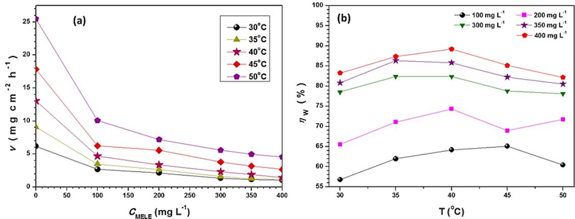
**Figure 3:** (a) Corrosion rate of carbon steel immersed in 0.5 M H<sub>2</sub>SO<sub>4</sub> as a function of the concentration of MELE and (b) effect of temperature on MELE efficiency
