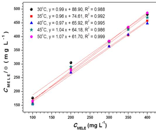
**Figure 8:** Langmuir isotherm applied to the adsorption of MELE compounds on the carbon steel surface
