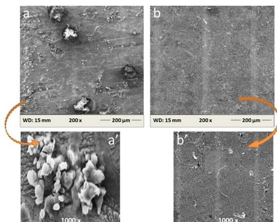
**Figure 6:** SEM image of the carbon steel after 1 hour of immersion in 0.5 M H<sub>2</sub>SO<sub>4</sub> (a) without and (b) with 400 mg L<sup>-1</sup> of MELE
